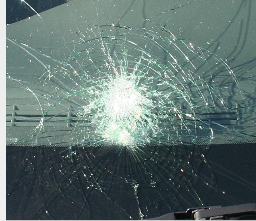
Windshield cracking typical of laminated safety glass
