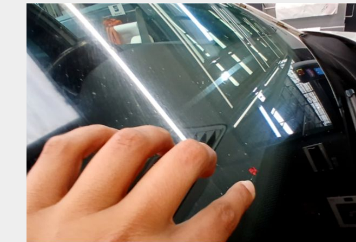
Chip damage detection
