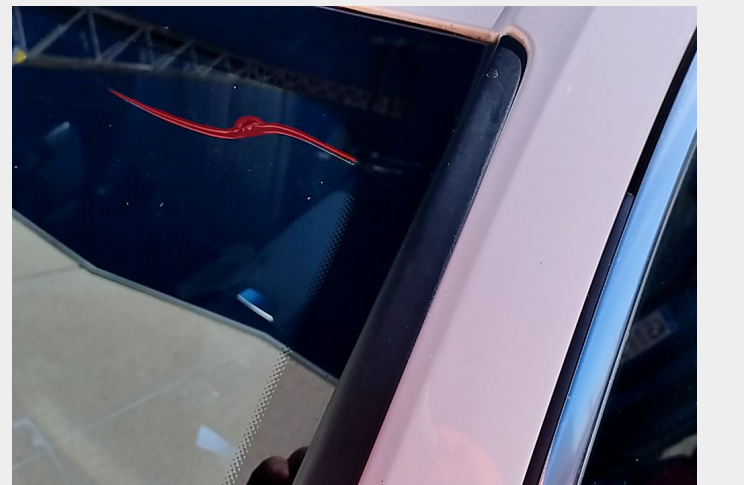
Bullseye and crack damage detection
